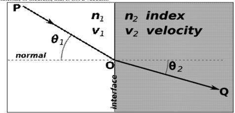
More precisely, the refractive index is constant for any given pair of materials, and can be defined as
