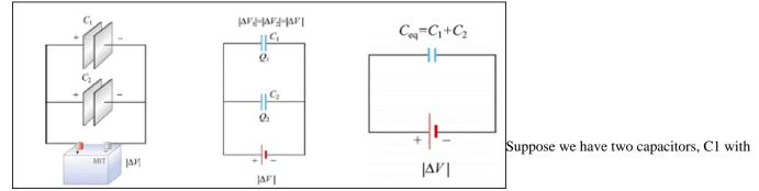
charge  $Q_1$ , and C2 with charge  $Q_2$ , and that they are connected in parallel, as shown in the figure above. The left plates of both capacitors  $C_1$  and  $C_2$  are connected to the positive terminal of the battery and have the same electric potential as the positive terminal. Similarly, both right plates are negatively charged and have the same potential as the negative terminal.
