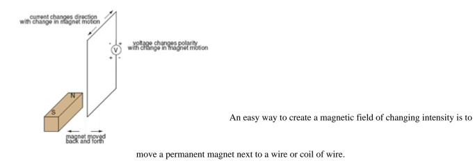
**Remember:** the magnetic field must increase or decrease in intensity perpendicular to the wire (so that the lines of flux "cut across" the conductor). Otherwise, no voltage will be induced.
