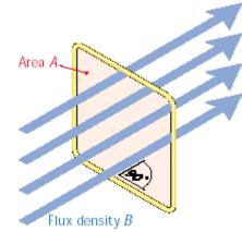
Magnetic flux can be thought of as the total number of magnetic field lines
