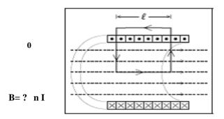
The magnetic field inside a solenoid is proportional to both the applied current and the number of turns per unit length. There is no dependence on the diameter of the solenoid or even on the fact that the wires are wrapped around a cylinder and not a rectangular shape.
