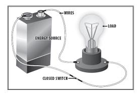
Complete path allowing electricity to flow from the energy source to the load
