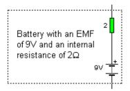
Internal resistance is a feature of all practical power supplies. Different battery designs will have different internal resistances, and the manufacturers will often take steps to minimize the internal resistance.
