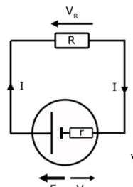
We can obtain important equations for E and r by considering a cell with resistance in a circuit.
