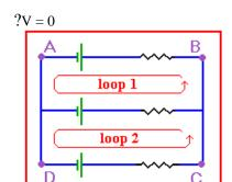
In Figure 1 the total voltage around loop 1 should aggregate to zero, as with the total voltage in loop 2. Furthermore, the loop which consists of the outer part of the circuit (the path ABCD) should also sum to zero.
