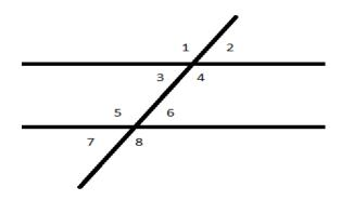
Pairs of angles in matching corners are called Corresponding Angles.
