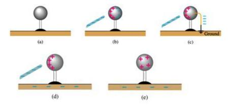
Charging a metal sphere by the process of induction.
