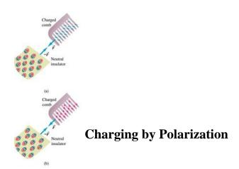
Although the charges (on the electrons) are tightly bound to the atoms in an insulator they are free to move slightly within the atom. This is called <u>polarization</u>.
