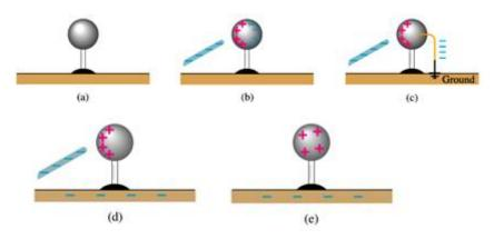
Charging a metal sphere by the process of induction.
