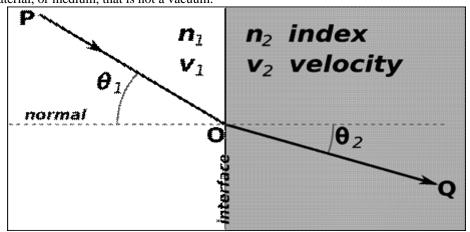
More precisely, the refractive index is constant for any given pair of materials, and can be defined as
