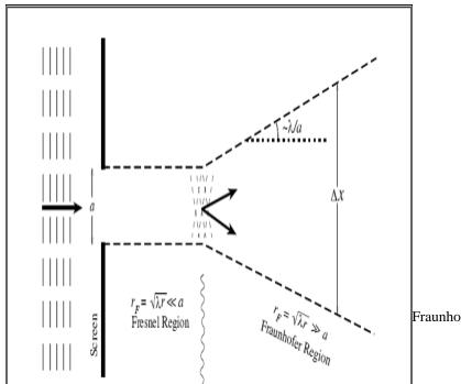
Fraunhofer diffraction occurs with plane wave fronts
