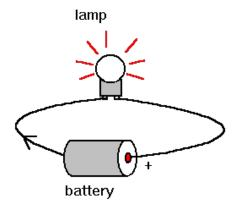
By definition, an electric current I is the amount of charge q flowing per second, hence I = q/t. Current is measured in Colombs per second (also called Amperes, see below). However, the charge on the electron is only a tiny fraction of a Coulomb -- hence a current of 1 Coulomb per second would correspond to an awful lot of electrons running around.
