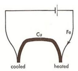
Jean-Charles Peltier found that when two metal wires of different materials were joined to form an electrical circuit and a direct electrical current was made to flow through the circuit, one junction would become cold and the other junction would become hot;
