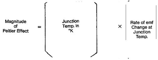
The Peltier effect is given as the product of the absolute temperature ("K") of the junction and the rate of change of the thermal EMF of the junction at that temperature. (Fig. 3) If a complete analysis were done, one would find that the Peltier effect produces no measurable change in the temperature of the junction when the only current through it is that due to the thermal EMF.
