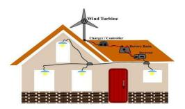
Wind turbines are more modern wind machines that use large blades to generate electricity. These machines consist of blades that are mounted on a turning shaft. The shaft has a gear transmission box that increases the speed of the blades. The transmission is attached to another shaft that turns a generator to create electricity. Wind turbines can be used for charging batteries, pumping water and powering homes.
