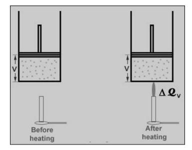
Consider a cylinder fitted with a frictionless <u>piston</u>. An ideal gas is enclosed in the cylinder.
