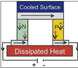
Thermoelectric cooling is a way to remove thermal energy from a medium, such
