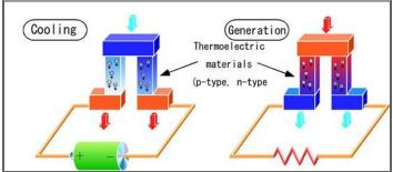
Thermoelectricity is a two-way process that may be
