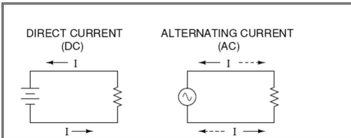
AC means “Alternating Current” and DC means “Direct
