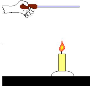
Objects undergo changes in dimension when they are heated. This change in length or area or volume is called "Thermal Expansion."
