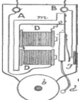
out through the metal of the armature, the contact screw, g, and the terminal B. Such a current
