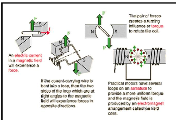
The general working mechanism is the same for all electric motors (see first figure above):
