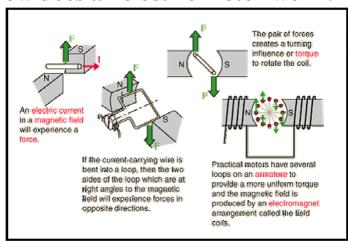
The general working mechanism is the same for all electric motors (see first figure above):
