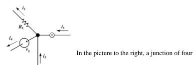
conductors (i.e. wires) is shown. The currents i2 and i3 are flowing into the junction, while i1 and i4 flow out of it. In this example, Kirchhoff's Junction Rule yields the following equation:
