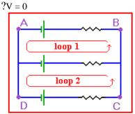
In Figure 1 the total voltage around loop 1 should aggregate to zero, as with the total voltage in loop2. Furthermore, the loop which consists of the outer part of the circuit (the path ABCD) should also sum to zero.
